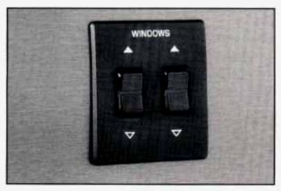
If you have optional power windows, the controls are on each of the front side doors. The driver's door has a switch for the front passenger window as well. Your power windows will not move unless the ignition has been turned to RUN.
